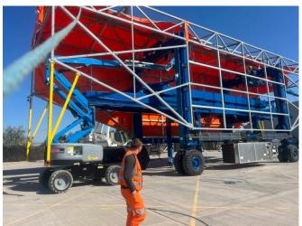
Wise Handling, based in Bradford, West Yorkshire, required a large, custom machine cover for a straddle carrier used by their client, Siemens. This carrier, designed to lift 60 tonne trains for maintenance and repair, needed a durable cover to protect ongoing work from the elements.
